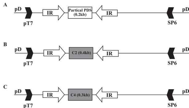
**Fig. (1).** Illustrations (not to scale) of the various IR-X-RI satellites. **A.** IR-PDS-RI. **B.** IR-C2-RI. **C.** IR-C4-RI. pD denotes pDRIVE plasmid sequences. pT7 and SP6 denote the positions of the respective promoters.
